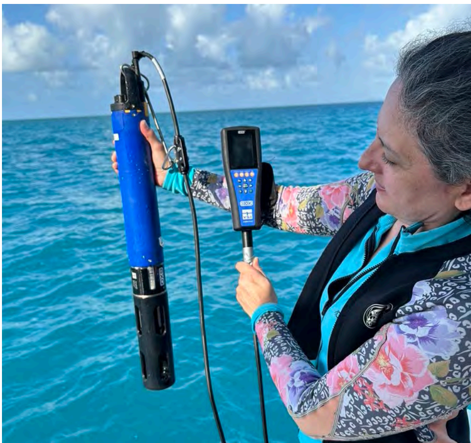
Figure 5. Additional water column data collected onboard the mothership using a hand-held sonde (Xylem - YSI EXO2 Multiparameter water quality sonde).
